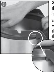
3) Fit the flange onto the rim of the bowl. The ribs of the flange should be lined up with the flat panel of the bowl. Check that the flange is correctly fitted.
