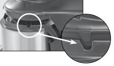
Make sure that the pin on the motor shaft is correctly lined up with the corresponding notch in the basket hub.
